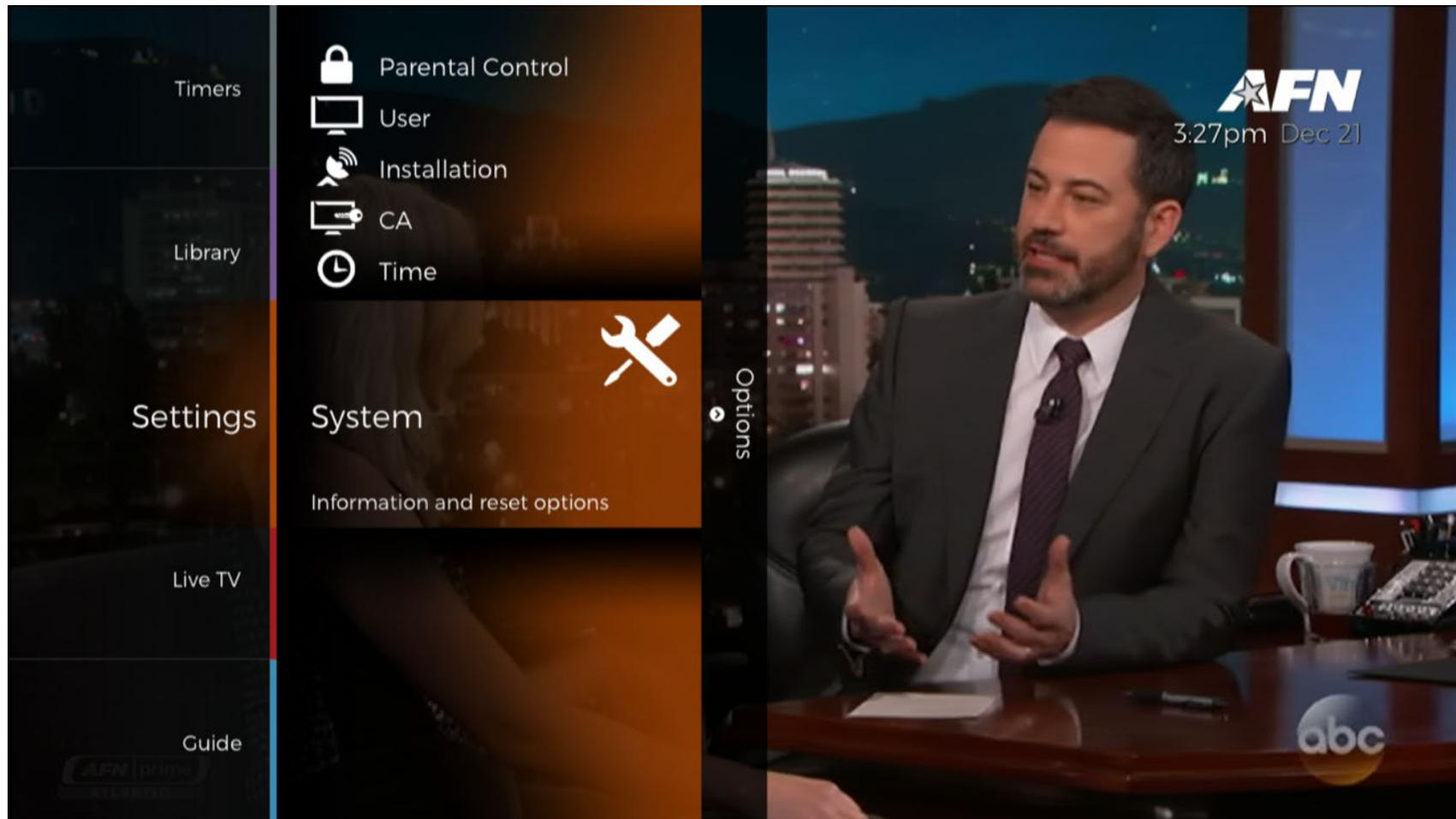
The **'System'** submenu is where **'System Info'** can be viewed as well as options to reset the Decoder to **'Factory Default'** and **'Change PIN'** for the system PIN number.
